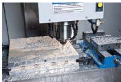
Below: This series of six photos illustrates a machining time of 11 minutes from start to rough-cut core features. QC-10 mold alloy is ideal for lights-out machining and boosting process efficiency.
