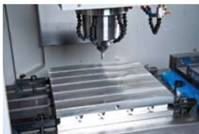
Below: This series of six photos illustrates a machining time of 11 minutes from start to rough-cut core features. QC-10 mold alloy is ideal for lights-out machining and boosting process efficiency.
